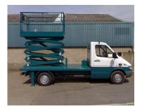
1B – Rider and Pedestrian Electric and ICE – Static Boom - This machine can be driven into position but cannot be moved when the carrier is elevated.
