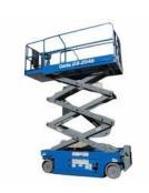
3B – Rider – Electric and ICE – Mobile Boom - This machine can be driven into position and driven when the carrier is elevated.
